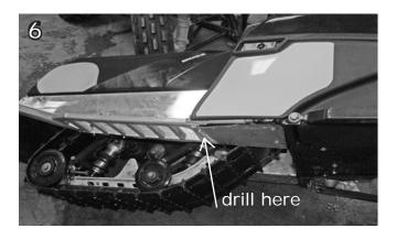
Tip sled on side. Drill from bottom through the rolled lip into the finger of the front of the Sled Tread with a 3/16" bit and rivet with 1 rivet as noted in picture above.
