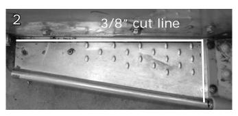
Measure 3/8" out from tunnel on existing running board and 3/8" back from angled foot rest and mark a line. You should be marking just inside the dimples on the existing boards.
