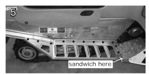
Put new running boards into front rolled edge and sandwich the new Sled Treads between the plastic and the running boards. Make sure that the new running boards are pushed down against the 3/8" lip and are pushed fully down on the lip of the tunnel. Drill (2) 3/16" rivet holes in the front using existing holes as a guide, and secure with (2) large head rivets.
