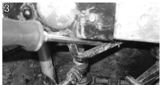
Note: On stock suspension – pry inward on torsion spring to prevent cutting spring. Cut off old running board with saw or cutoff wheel. You may need to grind slightly around bumper.
