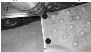
Drill out 2 rivets at bottom of plastic foot rest
