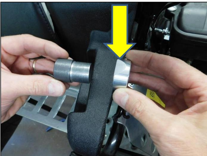
Make sure the flat spot on the retaining collar is at the 12 o'clock position.
