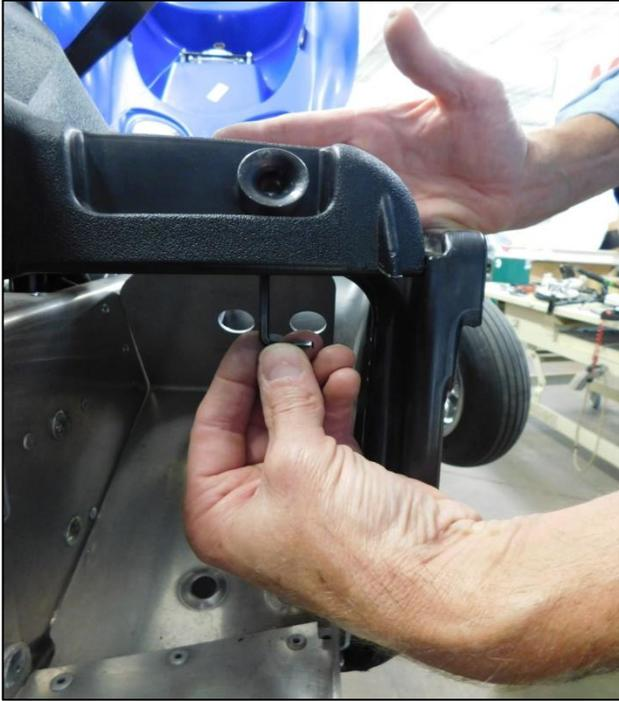
Use a 5/32 allen wrench to tighten the set screw to hold the collar.
