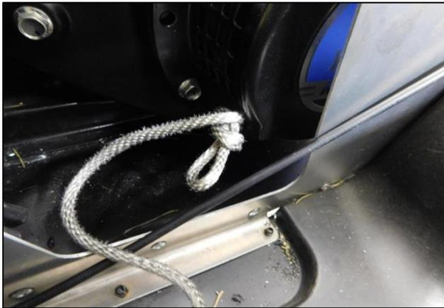
Pull starter cord to the end of travel & tie a secure knot next to recoil. This will prevent the cord from pulling all the way into the recoil when the handle is removed.
