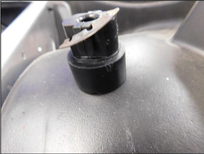
Using a screw driver pry the retainer from the back of the OEM starter bushing until it is completely removed. Then remove the bushing from the sled.
