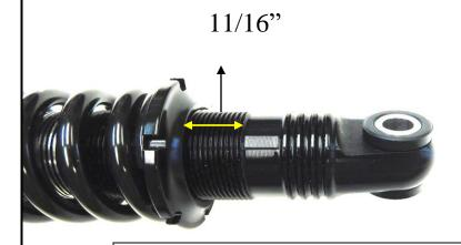
ADJUSTING SPRING RETAINER PAST THE ABOVE MEASUREMENT WILL CAUSE SHOCK DAMAGE.
