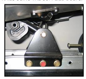
POLARIS: YOU WILL NEED TO DRILL A 5/16 HOLE IN THE RAIL IN THE LOCATION SHOWN BELOW AND INSTALL THE BOTTOM OF THE RACERIDE BETWEEN THE RAILS USING THE SUPPLIED BOLTS.
