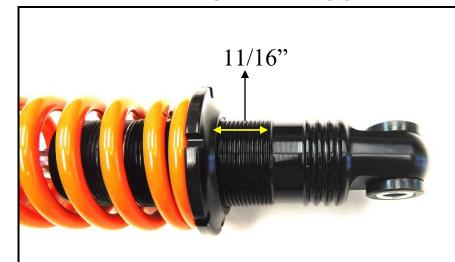
ADJUSTING SPRING RETAINER PAST THE ABOVE MEASUREMENT WILL CAUSE SHOCK DAMAGE.
