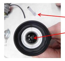
USING 6MM SOCKET OR NEEDLE NOSE PLIERS PUSH DOWN AND \_\_TURN PLASTIC NUT TO REMOVE NEEDLE
