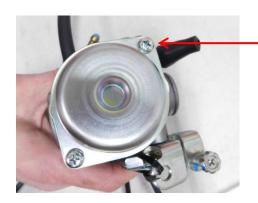
USE A GOOD PHILLIPS SCREW DRIVER TO REMOVE SCREWS. (SCREWS WILL BE TIGHT)
